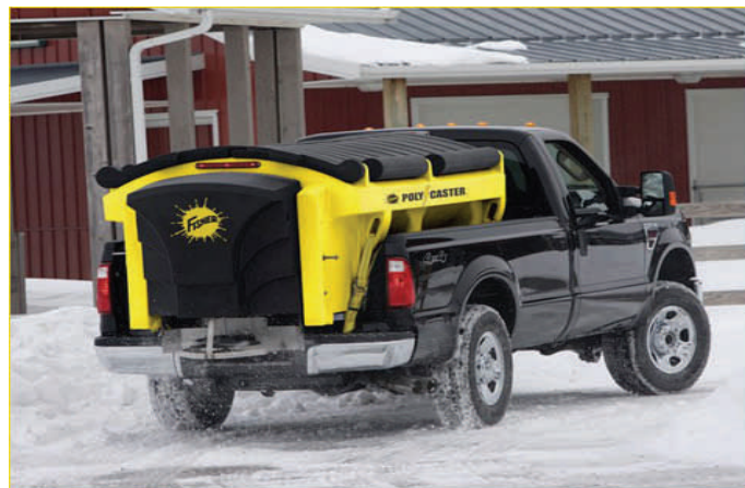
Poly spreaders with electric motors are proving to be the future of salt spreading technology.
